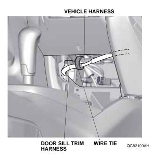
20. Route the door sill trim harness as shown. Align the green tape on the door sill trim harness with the vehicle wire tie, and secure the door sill trim harness to the vehicle harness with one wire tie.
