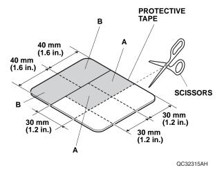
24. Attach masking tape to the vehicle panel at the measurement shown.
