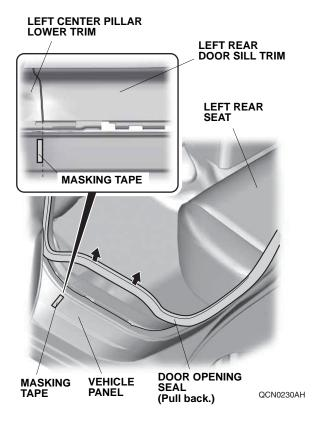
57. Peel back the ends of two adhesive backings on the left rear door sill trim and attach them to the front of the trim with masking tape.
