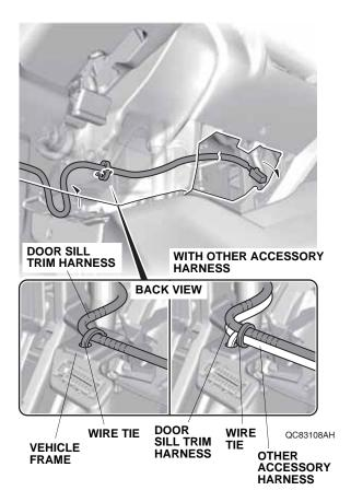
19. Secure the door sill trim harness to the vehicle harness with one wire tie.
