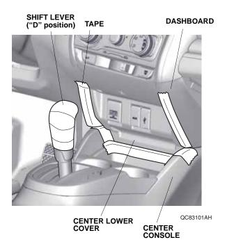
9. Remove the center lower cover, and unplug the vehicle connectors.
