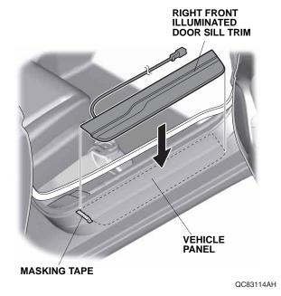
26. Using a felt-tip pen, mark the door opening seal and vehicle panel as shown.
