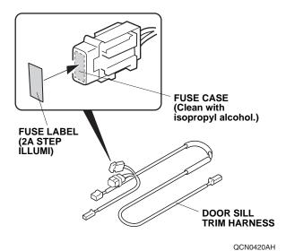
11. Attach the fuse label to the door sill trim harness fuse case.
